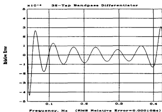
Fig 4. 32-Tap Bandpass Differentiator Filter Fit Error.
