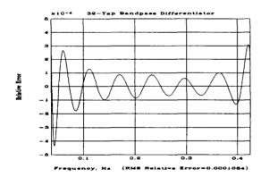
Fig 4. 32-Tap Bandpass Differentiator Filter Fit Error.
