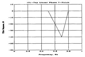
Figure 1. 101-Tap Asymmetric V-Notch Filter Amplitude Response.
