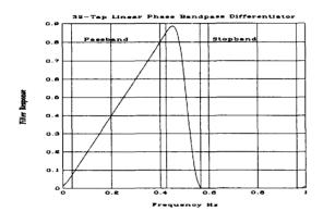
Fig 3. 32-Tap Bandpass Differentiator Amplitude Response.
